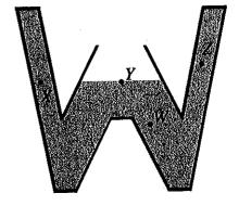
3. A U-tube is partly filled with water. Oil is then poured on top of the water on one side. The final water levels on both sides are as shown. The surface of the oil is not shown.
