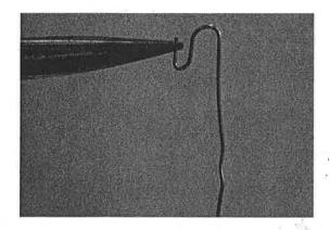
8. Use the pliers to bend a small portion of the paper clip upward to form a small U-shaped channel for the armature to sit in. Repeat this activity for the second paper clip.
