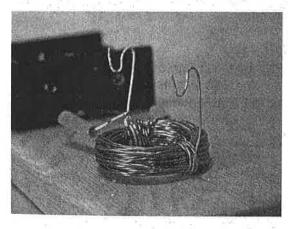
10. Bend the wire supports for the motor into a sideways S shape. To get this shape, bend the top inch of both wires down toward the base. The next step is to bend the last ½ inch of these wires back up again as shown in the picture. Both of the U-shaped slots should be at the same level or the motor will slide toward the lower side.
