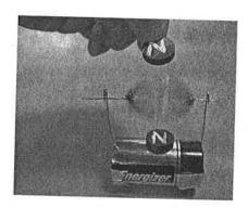
Another part of this demonstration shows a method for improving the efficiency of this motor. This requires a second magnet to increase the magnet field near the coil. Have students hold the second magnet about ½ inch above the spinning coil. When the coil is energized, it will push against both magnets. If the magnet is held close enough, a student can feel the force applied between the magnet and magnetized coil.
