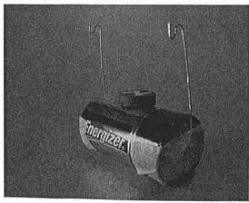
10. Both paper clip supports should have the bend at the same height, or the armature will fall off the support as it is spinning. The magnet is placed directly on top of the battery; it should be centered between the 2 paper clips. A piece of tape can be used between the battery and the table surface to keep the battery from rolling over during its operation.
