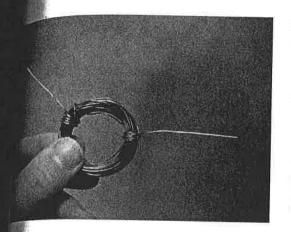
Take one of the ends of the wire and wrap it 3 or 4 turns around the coil of wire to hold it together. Tuck the end of the wire under one of the turns and then loop it around to knot it in place.
