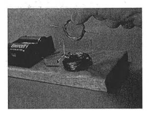
15. With the coil scraped and finely balanced, it is ready to run. Put the batteries in place, lay the coil down into the slots, and give it a spin.
