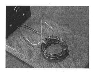
8. Cut an 8-inch piece of wire from the leftover supply. This wire has been painted white to make it easier to identify it in the pictures. The separate white wire is wrapped around the coil directly opposite from the right side support. Three inches of white wire extend up from the coil. This will form the left side support. The white wire is wrapped around the coil 3 or 4 turns and then tucked under one of the previous turns; this will knot it and hold it in place.
