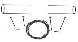
Hans Oersted's (1777–1851) famous discovery showed electricity could form magnetic fields and that the direction of the lines of force radiates perpendicular from the wire. Students can build a tangent galvanometer to show the magnetic field produced by coil and battery.
