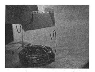
2. Glue the coil to the wood base. Use a silicone adhesive and apply it liberally to the bottom of the coil. Set the coil down onto the wood base in the intended position, and then press lightly to spread the glue onto the wood surface.
