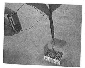
Sometime in every student's education, he or she should experiment with an electromagnet. A large nail wrapped with wire, a battery, and a box of paperclips allows students to explore magnetism and its properties.
