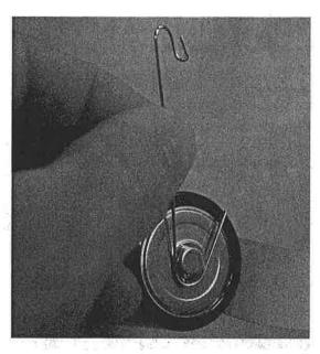
9. Use a few pieces of masking or plastic tape to hold the whole motor together. Tear off a 2-inch portion of tape and use this to attach the first paper clip to the side of the battery. The little knob on the battery should fit into the V portion of the paper clip. Position the second paper clip on the opposite side of the battery using another piece of tape.
