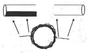
The coil is going to be supported on 2 bent paper clips. To make these holders, start by unbending the center portion of both paper clips. Try to straighten out the center of the clip as much as possible.
